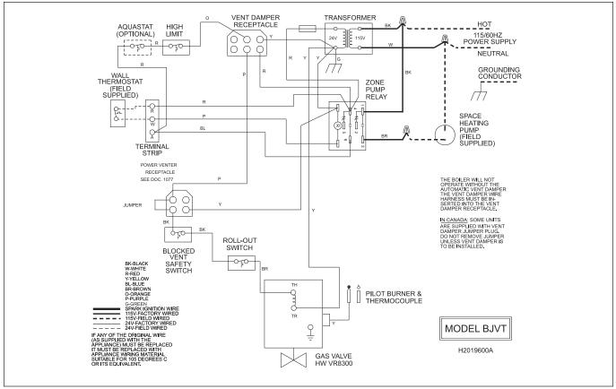
Figure 9c. Wiring Diagram, Standing Pilot System (BJVT).
